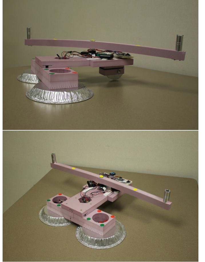
FIGURE 2. A physical Chaplygin beanie constructed primarily from one inch-thick extruded polystyrene foam. In place of casters, the aluminum pie plates hover on cushions of air generated by counter-rotating ducted fans to support the forward end of the cart with minimal friction between the cart and the ground. Batteries contribute significantly to the inertia of the cart; the rotor's large diameter helps to increase its rotational inertia without increasing the system's mass overall.
